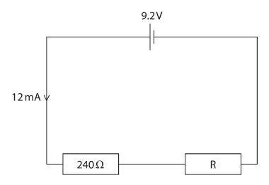
Calculate the voltage across resistor R.
