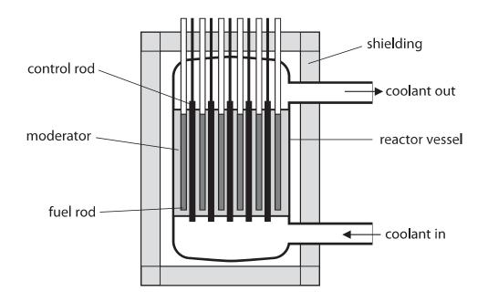
Each part of the nuclear reactor has a function and is made of a suitable material for its function.
