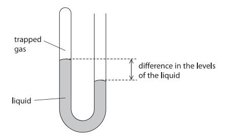
(a) One side of the manometer has some trapped gas. The other side is left open to the atmosphere.
